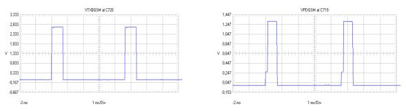
check VTXLOGSM at R709. Signal/amplitude is the same as VTXBGSM, but it is only present in PA-free and -low mode.
