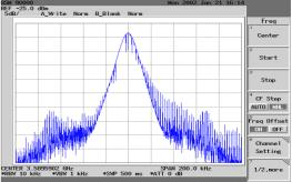
If no signal is measurable at T650 check VR7 2.6VDC at C650. If OK, set span of your analyser to e.g. 250MHz to check if the oscillator works on any other frequency as on the supposed. If this is the case check control voltage at C652 which normally is 2.1VDC on channel 37. In case of noise on the control voltage especially check C653 (tendency to leak). If the oscillator does not work at all, change G650 and retest the phone.
