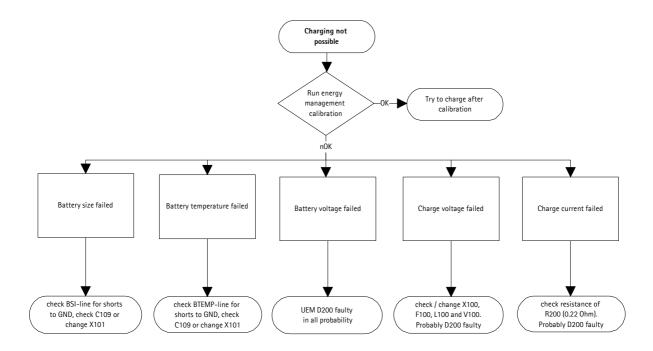
First thing you should do in case that charging of battery is not possible is to run energy management calibration. Note that calibration only works with JBV-1. In Service jig it is not possible because of missing bottom connector 1009.
