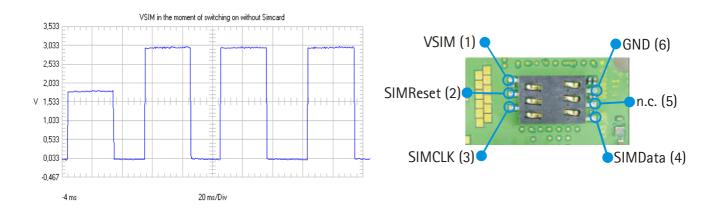
In case that the above mentioned signal is not measurable at one or more similares, check SIM lines for shorts to ground. Resistance of simdata- and VSimline normally is >  $200k\Omega$ , resistance of SIM reset- and SIM clock line normally is ~  $4.5M\Omega$ . If resistance of any line is not ok check parts the SIM lines consists of (R388, C203, C389).
